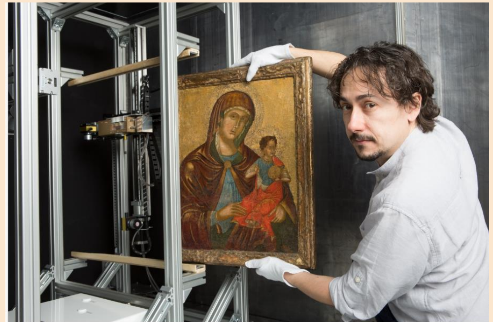
Slotting a painting into the X-ray scanner, which will analyse it at a high resolution. (Image: InsightArt s.r.o.)
